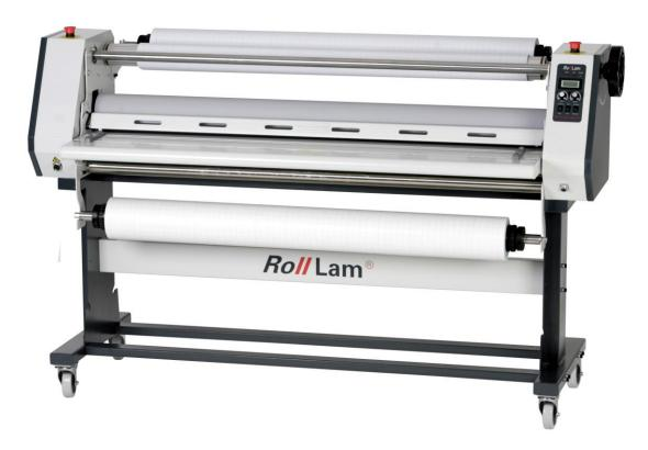
The upper roller of the models *Roll*Lam 120W, *Roll*Lam 140W and *Roll*Lam 160W is equipped with a thermoelement what makes it possible to heat the silicone roller to approx. 30°C-60°C.
